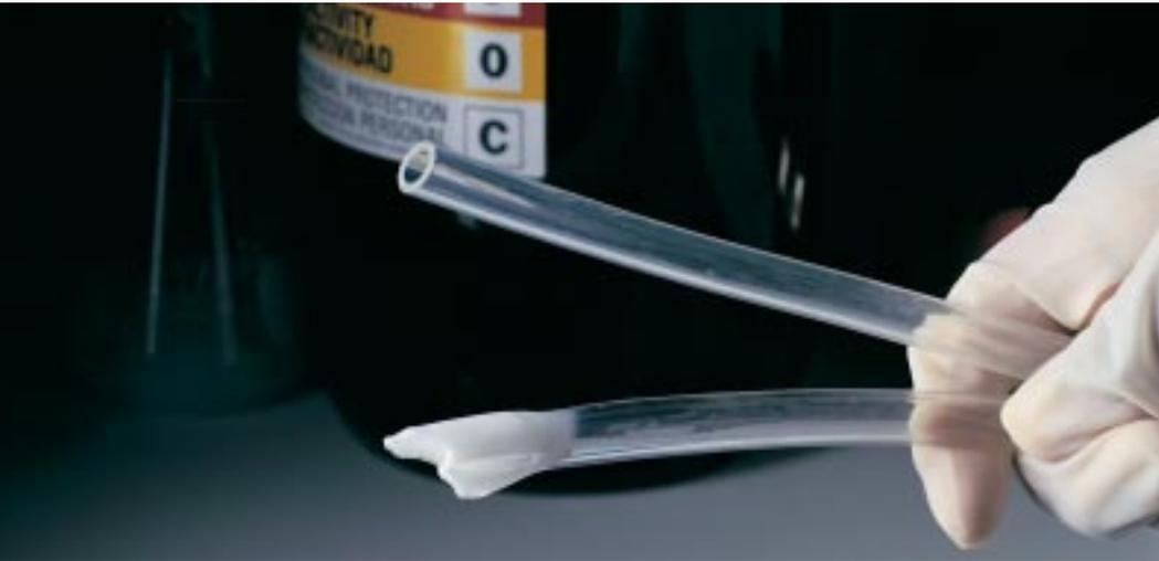
After being immersed in aggressive MEK for 16 hours (plus 4 hours drying time), Tygon® 2075 Ultra Chemical Resistant Tubing is still clear and flexible while PVC tubing is completely degraded and rendered useless.
